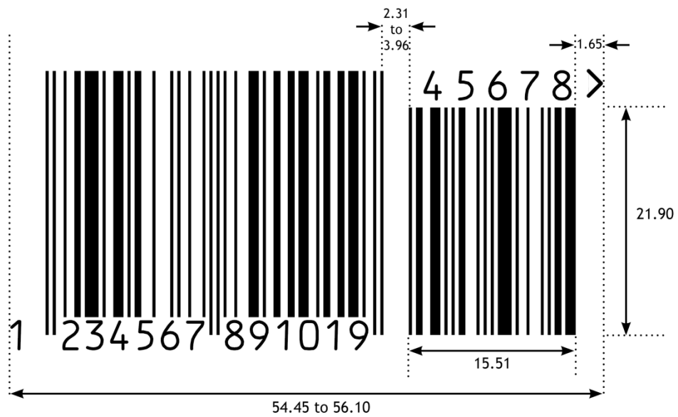
Figure 5.2.6.6-6. EAN-13 barcode with five-digit add-on symbol
