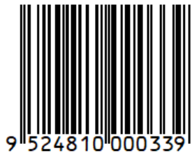
Figure 4.14-5. Example of EAN-13 with EAN/UPC HRI format
