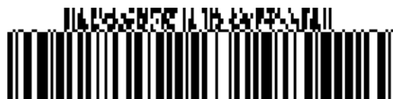
Figure 5.11.8-9. GS1-128 symbol with a four-column CC-A
