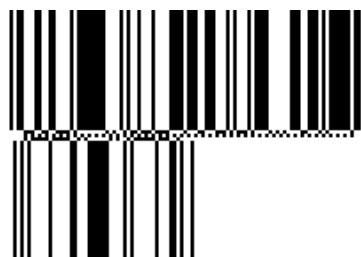
Figure 5.5.2.3.2-1. GS1 DataBar Expanded Stacked barcode
