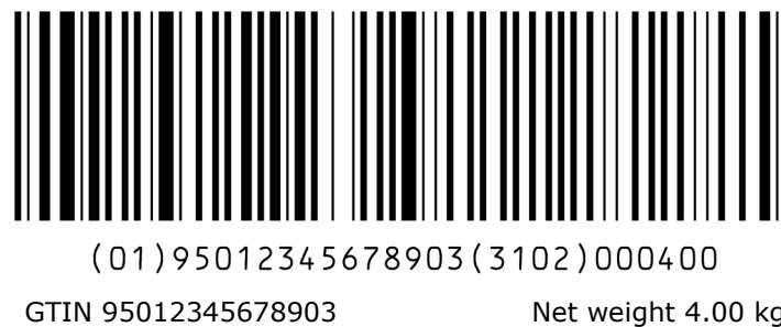
Figure 7.8.6.1-2. Data encoded in one concatenated GS1-128 symbol
