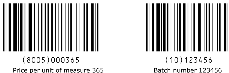
Figure 7.8.6.2-1. Data encoded in two GS1-128 symbols
