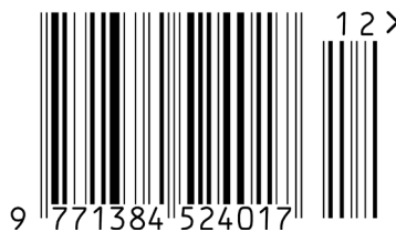
Figure 5.2.2.5.1-2. EAN-13 barcode with two-digit add-on symbol
