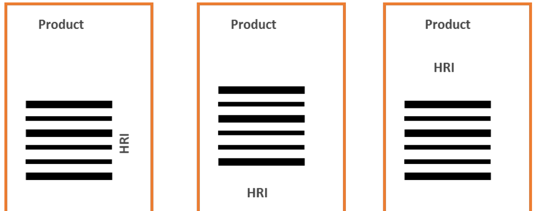
Figure 4.14-2. Locations of HRI for barcode in ladder orientation
