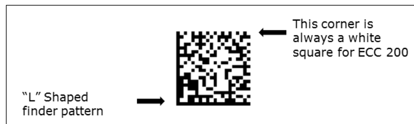
Figure 5.6.2-1. GS1 DataMatrix symbol
