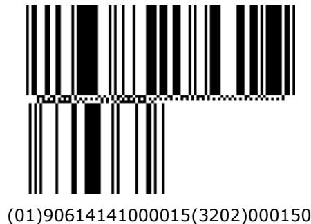
Figure 7.8.6.3-1. Example of GS1 DataBar Expanded Stacked barcode that uses concatenation
