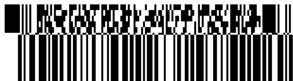
Figure 5.11.2-2. GS1-128 Composite symbol with CC-C
