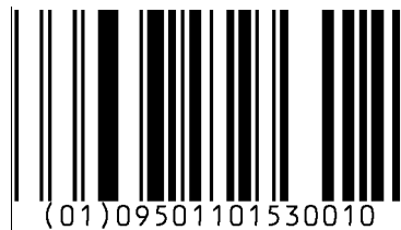
Figure 5.5.2.1.1-1. GS1 DataBar Omnidirectional barcode
