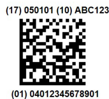
Figure 5.1-6. GS1 DataMatrix barcode
