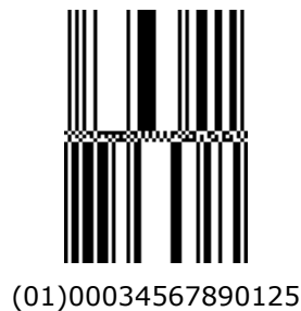
Figure 5.5.2.1.4-1. GS1 DataBar Stacked Omnidirectional barcode
