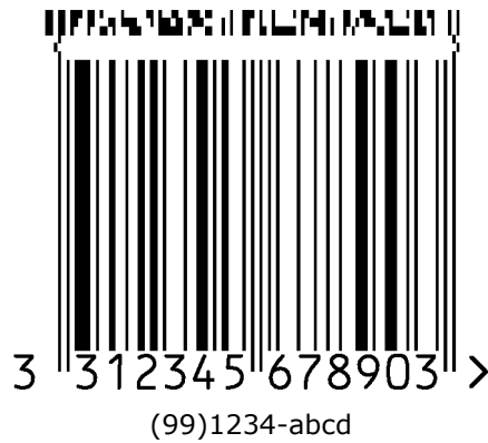
Figure 5.11.8-2. UPC-A symbol with a four-column CC-B component
