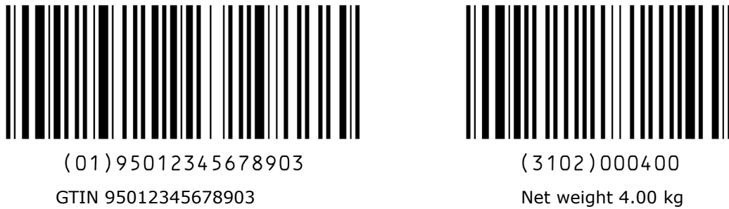
Figure 7.8.6.1-2. Data encoded in one concatenated GS1-128 symbol
